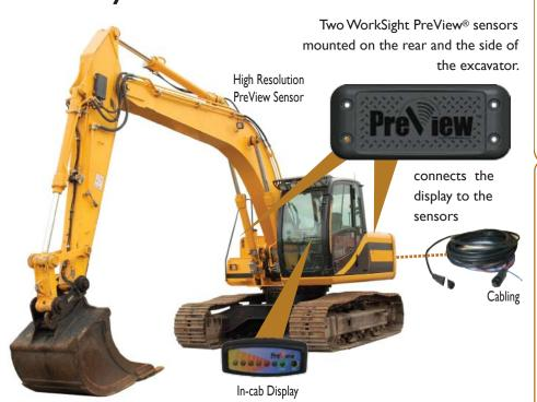
The display unit provides an audible and visual warning to the operator when an object or pedestrian is in the blind spot. This gives the driver extra time to react to prevent an accident.
