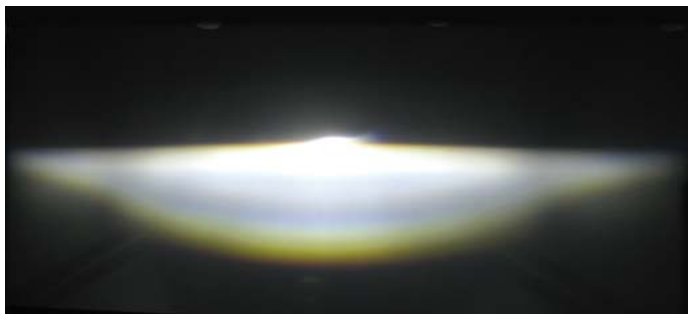
J.W. Speaker's DOT-Compliant Beam Pattern
