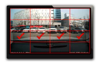
Continuously records at 1FPS (one frame per second). Videos are played back at 30FPS. 1-minute Time lapse Parking Mode video = 30 minutes real time coverage. Cover a period of more than 54 hours on a 32GB microSD card front and rear at the highest (Extreme) quality setting. When an impact is detected, the dashcam creates a buffered Event video.
